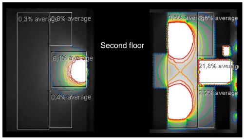
Figure 2. Daylight performance (daylight factor) for the room on first and second floor in the existing (left) and renovated (right) situation.
